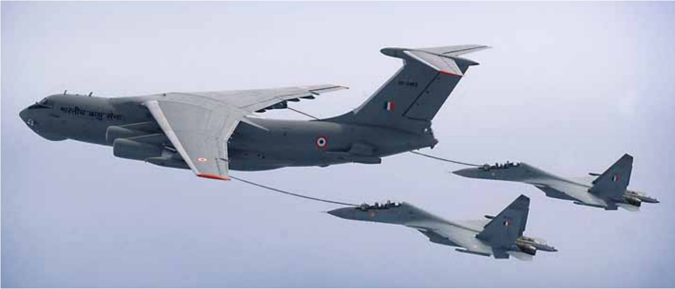
IAF's Su-30 aircraft being refuelled by IL-78 refueller
