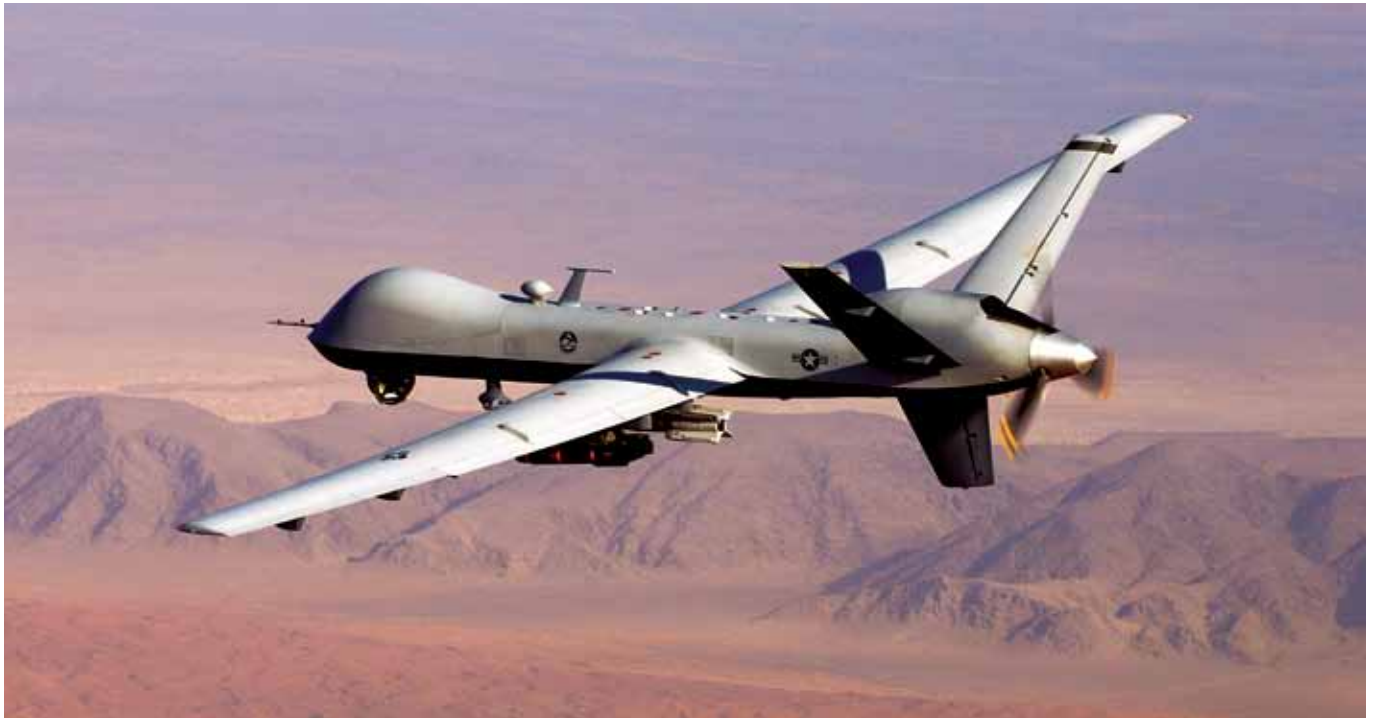
General Atomics MQ-9 Reaper armed with GBU-12 Paveway II laser guided munitions and AGM-114 Hellfire missiles
